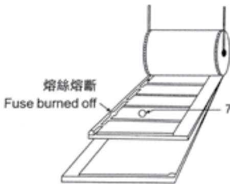
Figure 2. Fuse burned off on failure area
